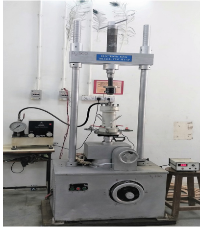
Fig. 8. Electronic rock triaxial setup
